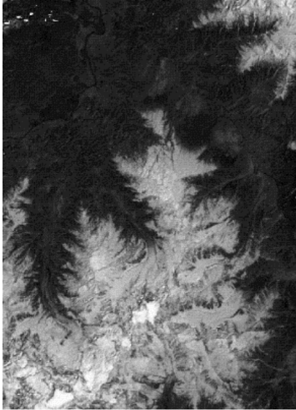
Fig. 6. Normalized SPOT 3 NIR image using the Minnaert-correction method (globally computed k ). Spectral variance visually appears to be reduced, however, extreme radiance values are found at the base of steep slopes.
